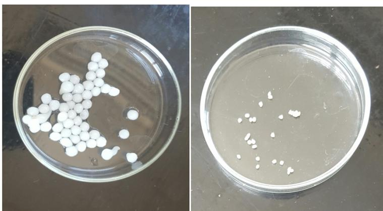
FIGURA: 8. ESFERAS PREPARADAS CON QUITOSANO HÚMEDAS (IMAGEN DE LA IZQUIERDA) Y SECAS (IMAGEN DE LA DERECHA)
