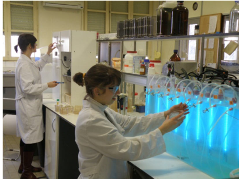
Figure 18: Installation for pasteurization of food with light Ultraviolet.
