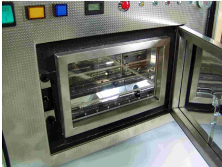
Figure 19: High intensity white light treatment chamber.
