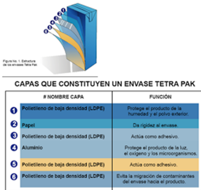
Fig. 5: Layers of material for cardboard packaging.
