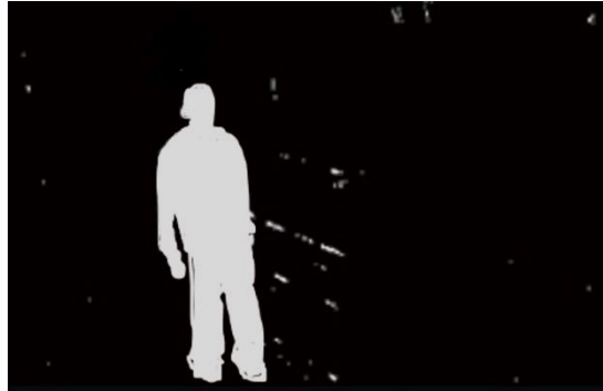
Figure 8. Background detection in OpenCv
