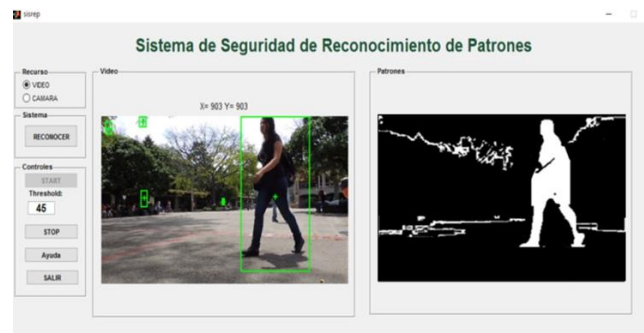
Figure 14. Object detection during the day with OpenCv.
