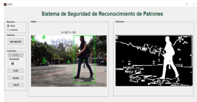
Figure 13. Detection of objects in the day with Matlab.
